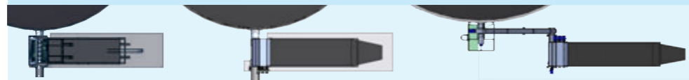
Storage capacity basic unit 10m 3 (with 4 attachment rings up to 13m 3 ). With push-off dosing unit: 35, 40, 45 or 50m 3
